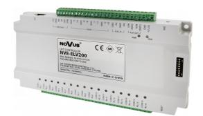
The lift controller realizes centralized management by connecting indoor monitor, outdoor panel and Wiegand card reader. With easy operation and setting, this device meets users' diversified needs. The module has two operating modes. The module relays can be connected directly to the elevator buttons or to the PLC inputs. Lift controller can be set to master and slave types. In one lift controller unit, the Master Controller communicates with other slave lift controller by RS485.
