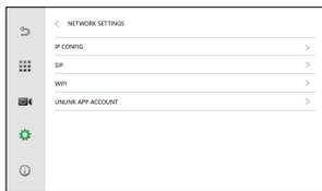
Select the WIFI option a window with the searched wireless networks will open. After selecting the network the authentication window will pop up, in the window enter the password to access the network then confirm with "Connect" button.
